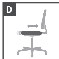
D. Seat slide mechanism — Seat cushion travels forward and back, then locks into position.
